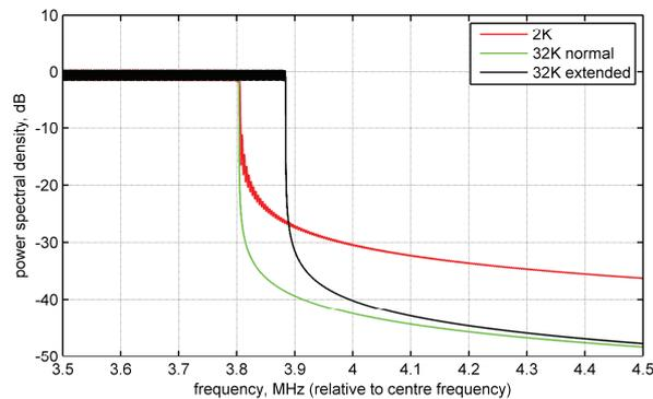
Because of its higher number of usable carriers the extended carrier mode has an increased data capacity as the normal carrier mode. Table 2.16 gives the gain of the extended carrier mode for the different FFT modes.
