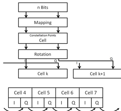
A cell is the result of mapping a later carrier. In contrast to DVB-T, mapping is not carried out after all interleaving processes but relatively early, after the error protection and after the bit interleaver. However, this is still followed by the cell interleaver, the time interleaver and the
