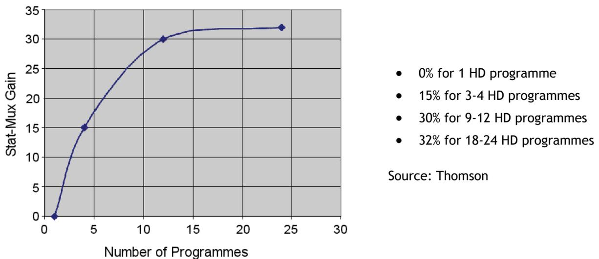
**Figure 4.11: Statistical multiplex gain with MPEG-4 AVC**
