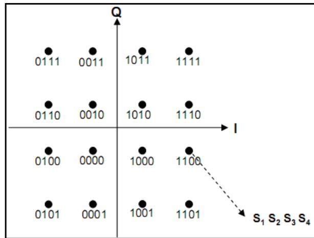
There are various ways of attributing the bits to the symbols. Best results are achieved if only one bit is changed when going from one symbol to the next closest symbol. In this way only one bit is mistaken when a symbol mismatch occurs with the next closest symbol. This coding is called Gray mapping. Figure 2.2 shows a Gray mapping constellation.
