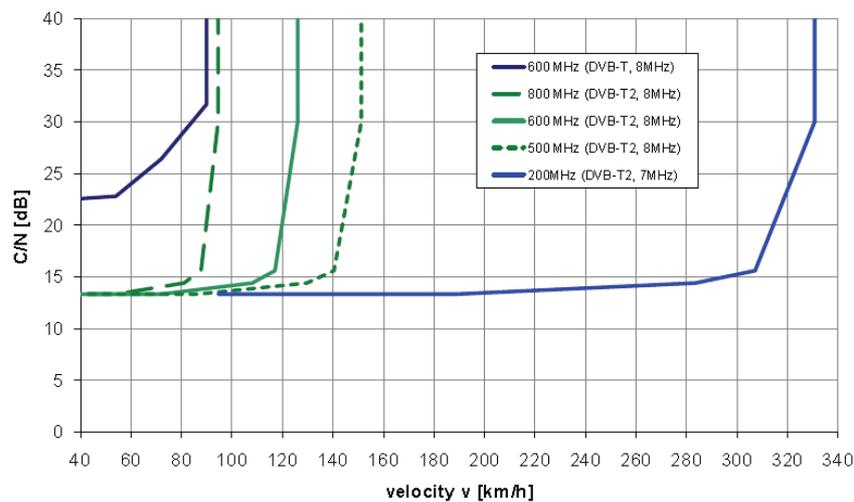
**Figure 2.5: Required C/N for DVB-T and DVB-T2 as a function of the velocity of the mobile receiver, 8k FFT (from [AFM2010])**
