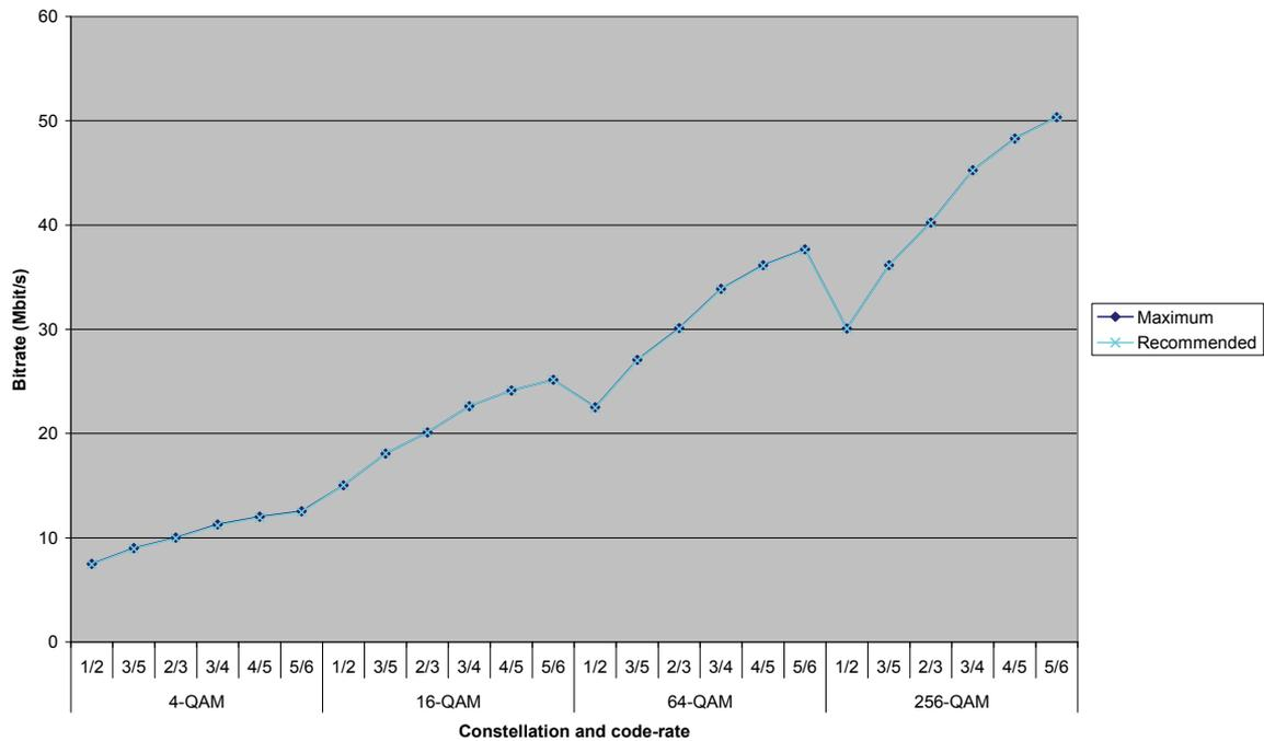
**Figure 2.1: Maximum bit rate and bit rate for recommended configuration with 8 MHz bandwidth and 32k PP7 (from [TS 102 831])**
