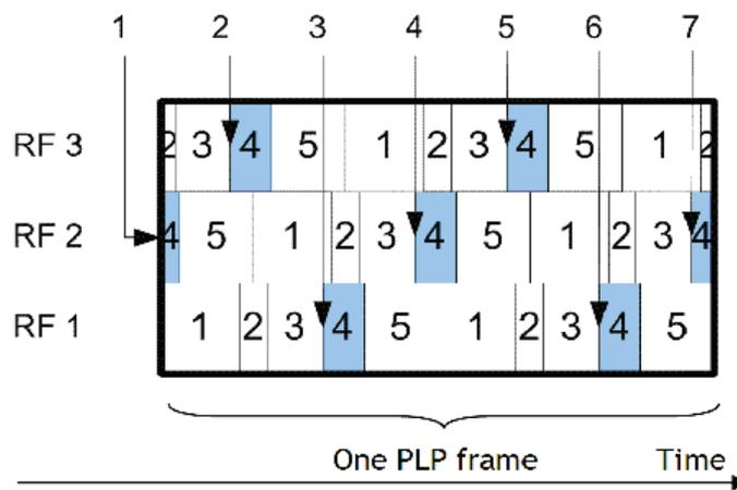
Figure 4.10: Example, TFS over three frequencies
