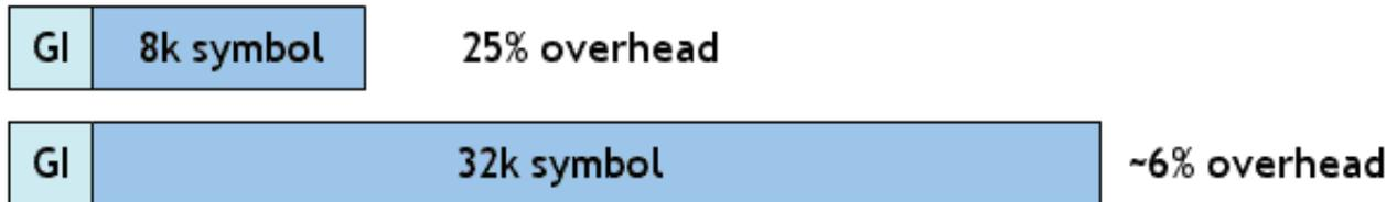
**Figure 2.8: Guard interval overhead reduction with larger FFT size (from [TS 102 831])**
