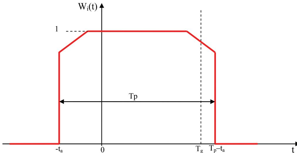
Figure 4.5: Weighting function  $w_i(t)$  (with an equalization interval EI starting at  $t = -t_a$ )
