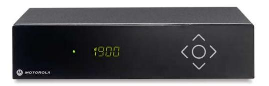
The Motorola VIP1900 series extends the possibilities for broadband television. Advanced video formats and decoding of High Definition television (HDTV) are supported in all models, whereas a built-in hard disk drive for PVR and a DVB-T receiver are available as options.
