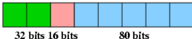
Figure 22.1. The anatomy of an IPv6 address
